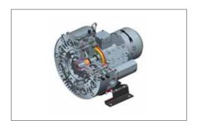
Blowers increase the pressure of the absorbed gas by a series of vortex motions formed by the centrifugal movement of the impeller. When the impeller is rotating, the channels in the impeller push the air forward by the centrifugal movement and a helical movement occurs. During this movement, the gas is continuously compressed along the channel and the pressure increases linearly. The pressurized air is transferred from the outlet duct of the blower to the installation to be used.
